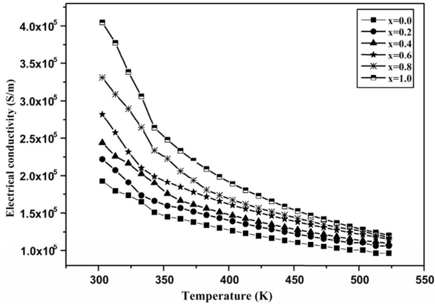
**Figure 3.** Electrical conductivity versus the temperature of the  $\text{Bi}_2\text{Se}_3\text{Te}_{3(1-x)}$  disks.
