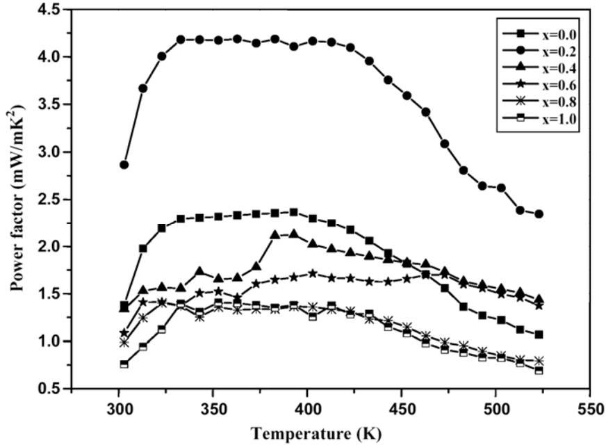
**Figure 5.** Power factor versus the temperature of the  $\text{Bi}_2\text{Se}_{3x}\text{Te}_{3(1-x)}$  disks.
