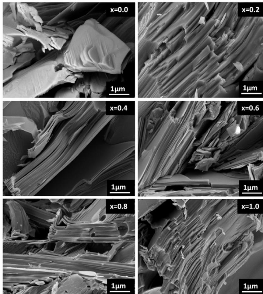
**Figure 1.** FESEM images of the  $\text{Bi}_2\text{Se}_{3-x}\text{Te}_{3(1-x)}$  ingots.
