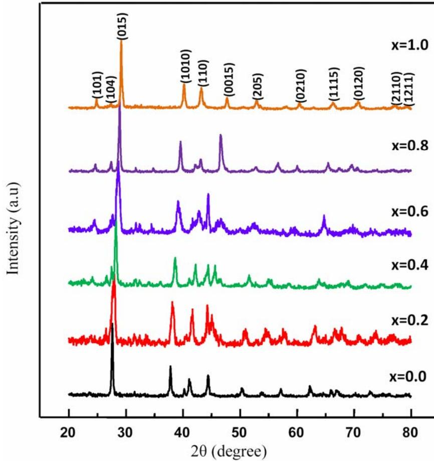
**Figure 2.** X-ray diffraction patterns of the  $\text{Bi}_2\text{Se}_3\text{xTe}_3(1-\text{x})$  powders prepared using rapid solid-state microwave synthesis.
