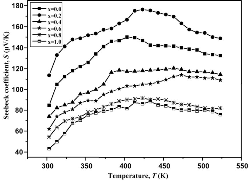
**Figure 4.** Seebeck coefficient versus the temperature of the  $\text{Bi}_2\text{Se}_{3x}\text{Te}_{3(1-x)}$  disks.
