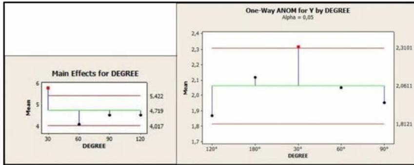
**Figure 9.** Analysis of variance at 5% level of significance by Minitab software 14 the effects of the degree in the amount of springback and in the aspect ratio of the grains of interstitial-free steel.
