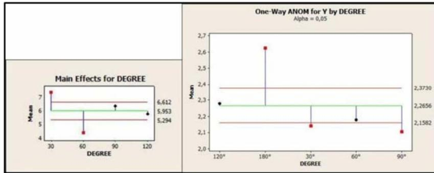
**Figure 5.** Analysis of variance at 5% level of significance by Minitab software 14 effects of the degree in the amount of springback and in the aspect ratio of the grains of low carbon steel.
