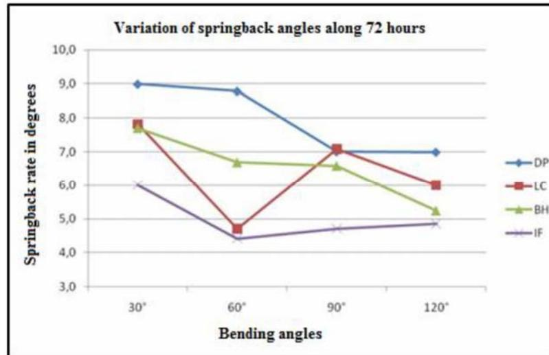
**Figure 2.** Angle variation of the springback effect for different bending angles after 72 hours.
