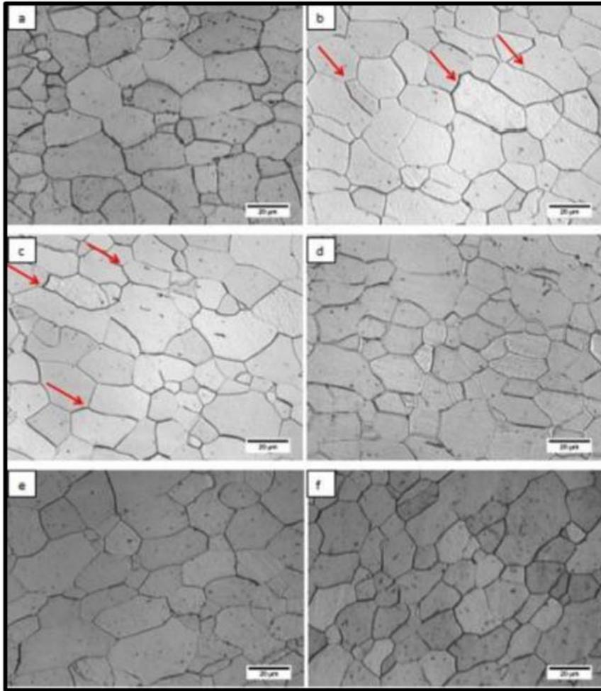
**Figure 8.** Optical microscopy images bake hardening steel as received and subjected to sheet metal forming, where (a): material as received, (b) and (c): 120°, (d): 90°, (e): 60°, and (f): 30°, increase of 500×, reagent Nital 2%.
