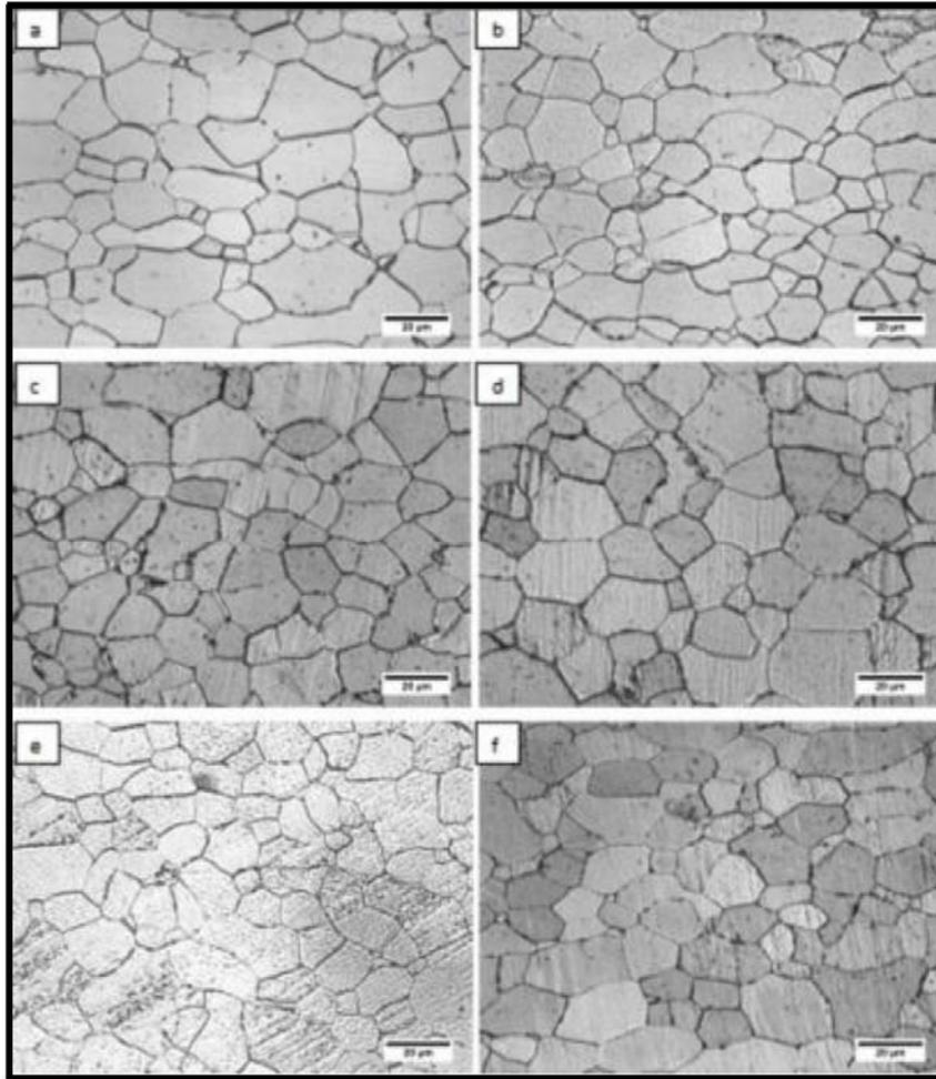
**Figure 6.** Optical microscopy images low carbon steel as received and subjected to sheet metal forming, where (a): material as received, (b): 120°, (c) and (d): 90°, (e): 60°, and (f): 30°, increase of 500×, reagent Nital 2%.
