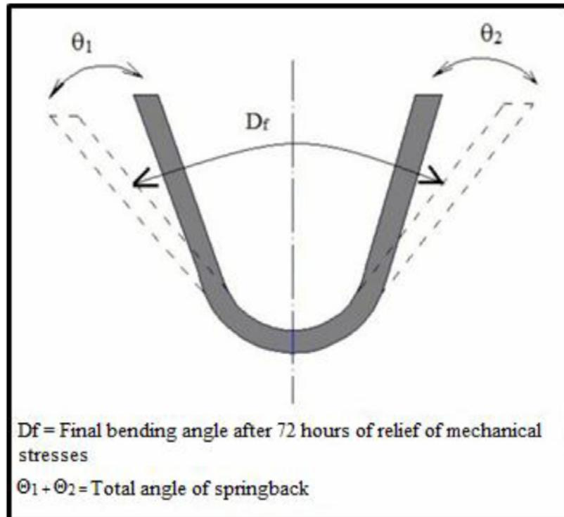
**Figure 1.** Representation of a specimen steel sheet undergoing to the springback effect.
