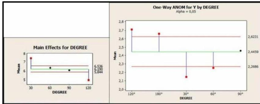
**Figure 7.** Analysis of variance at 5% level of significance by Minitab software 14 for the effects of the degree in the amount of springback and in the aspect ratio of the grains of bake hardening steel.
