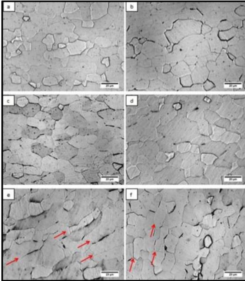
**Figure 10.** Optical microscopy images interstitial free steel as received and subjected to sheet metal forming, where (a): material as received, (b): 120°, (c): 90°, (d) and (e): 60°, and (f): 30°, increase of 500×, reagent Nital 2%.
