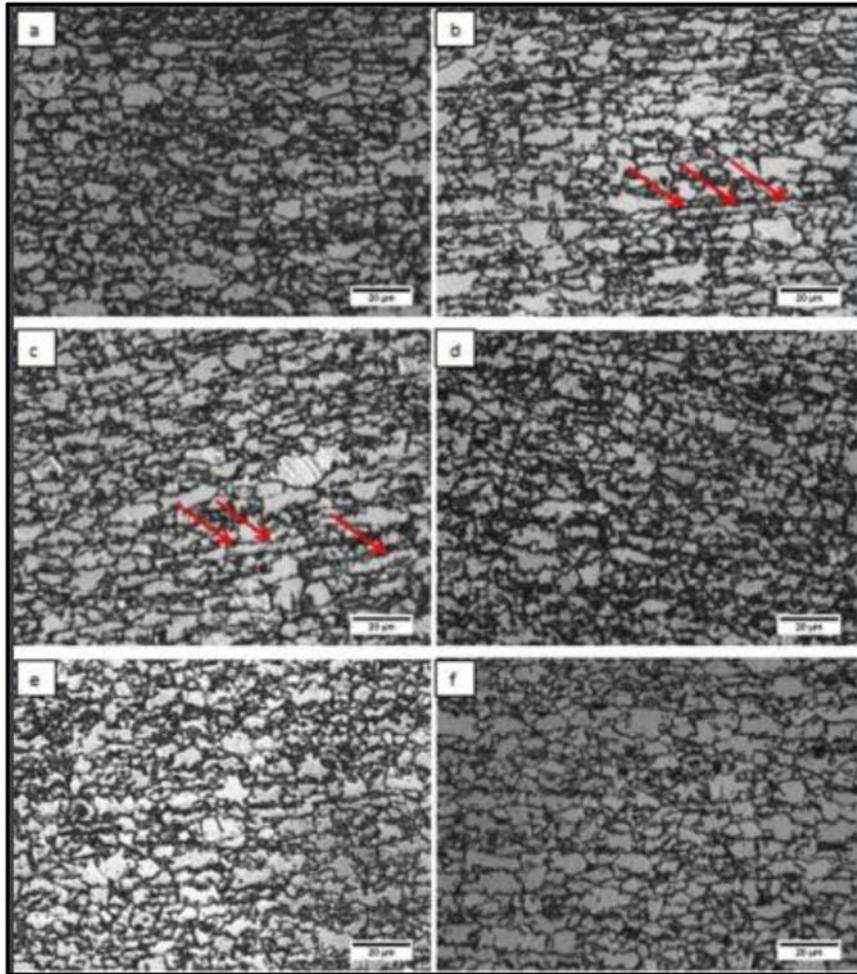
**Figure 4.** Optical microscopy images dual-phase steel as received and subjected to sheet metal forming, where (a): material as received, (b) and (c): 120°, (d): 90°, (e): 60°, and (f): 30°, increase of 500×, reagent Nital 2%.
